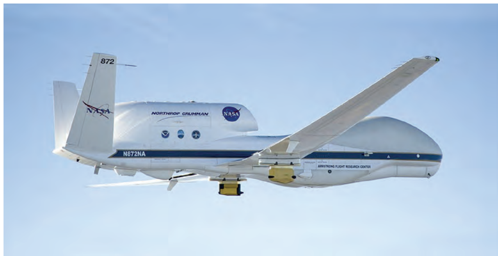
FIGURE 26 NASA Global Hawk shown with the CAST AITS and ATTREX Hawkeye instruments on the wing pylons.
