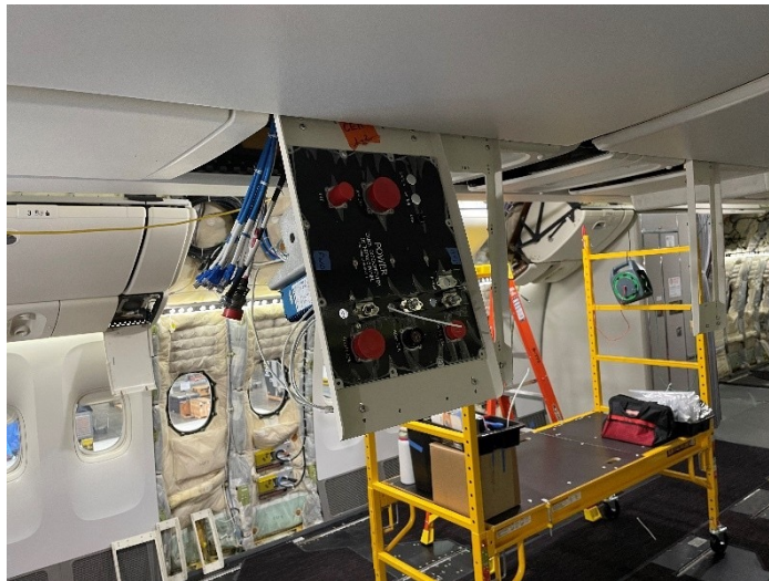
The new experimenter interface panel installed on the NASA B777. Credit: Derek Rutovic / NASA
