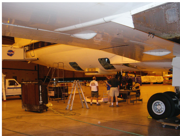
Figure 46: University of Kansas MCoRDS antenna system is integrated to the DC-8 in preparation for Antarctic Operation ICE Bridge mission.
