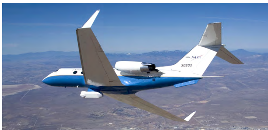
Figure 50. The AFRC C-20A flew SAR imagery missions for ASAR, Delta-X, and Earth Surface missions.
