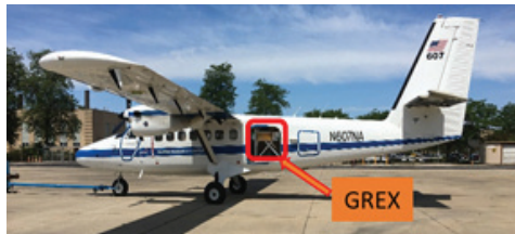
GREX mounted in NASA Glenn Twin Otter. Science flights were conducted with the cargo door off.
