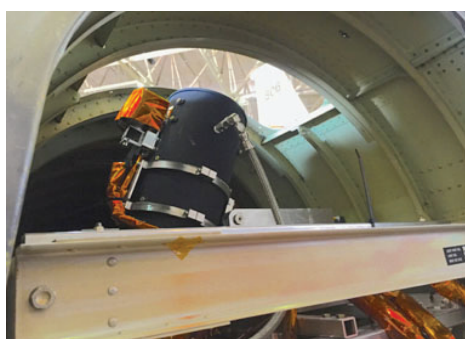
IRIS telescope on ARTEMIS mount in ER-2 wing pod tail
