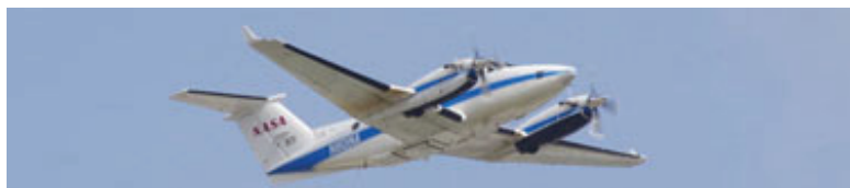
NASA 801 taking off from New Orleans' Louis Armstrong Airport with DopplerScatt onboard (conical radome mounted in the nadir-looking port of the King Air) for the science flight, March 26, 2018.
