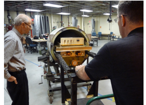
During a test phase for the PODEX experiment, engineers and the crew at Dryden Aircraft Operations Facility loaded the Research Scanning Polarimeter into the "superpod," for placement under the wing of the ER-2. Credit NASA/Matteo Ottaviani
