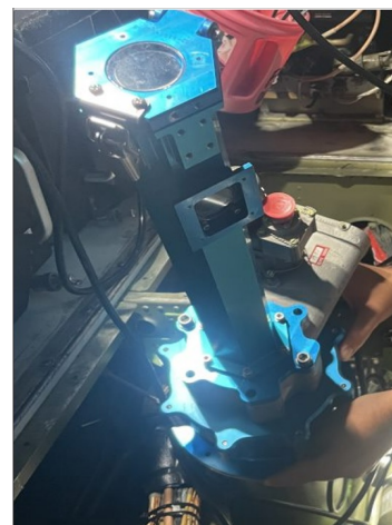
Launch tube installation on the LaRC G-III aircraft
