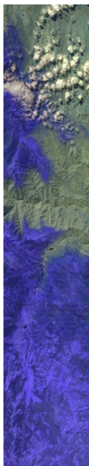
Figure 50. False-color short-wave infrared PICARD image over Yosemite National Park on March 31, 2023. Red, green, and blue channels are mapped to the 2.15, 1.55, and 1.15 micrometer wavelength PICARD bands, therefore snow appears deep blue, clouds appear white, and vegetation appears yellow green in the image.
