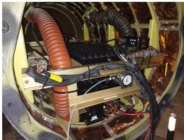
Figure 49. PICARD instrument installed in the ER-2 pod. Photo credit: NASA
